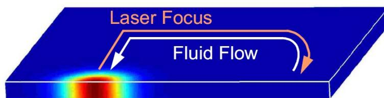
**Figure I.2:** Pumping water optically along arbitrary patterns. Fluid flow along the letters “LASER PUMP” is driven by dynamically heating a thin fluid film with a laser scanning microscope. As seen, complex flow patterns are easily accomplished. No channels restrict the fluid flow. Local pumping of the fluid film is the result of thermoviscous fluid movements for each passage of the laser focus. We visualize the water flow by fluorescent tracer particles.
