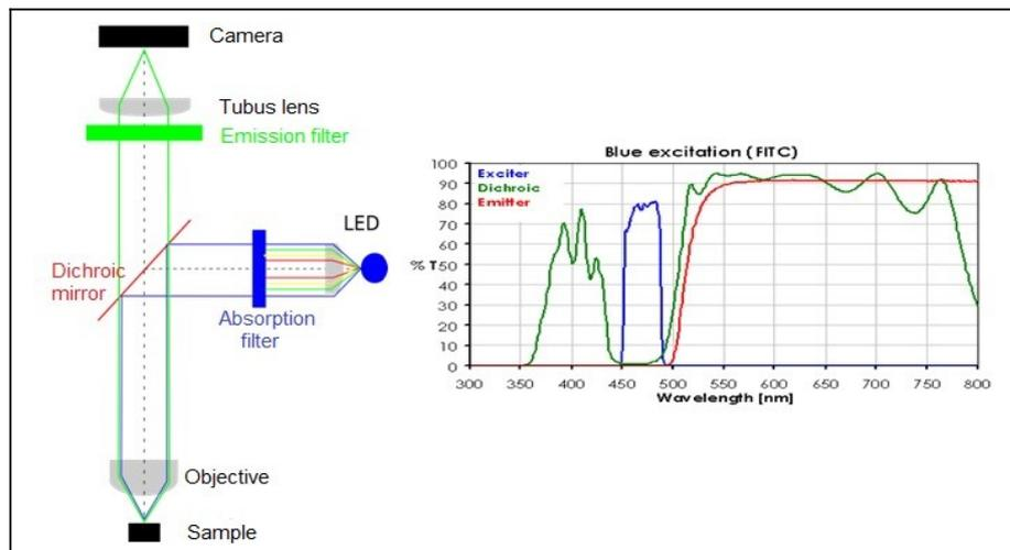
**Figure 3:** Left: Optical path of a typical fluorescence microscope;
