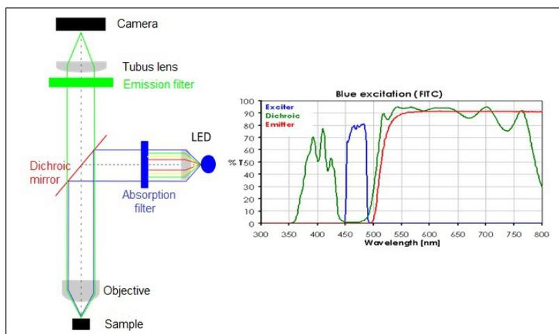
Figure 3: Left: Optical path of a typical fluorescence microscope;
